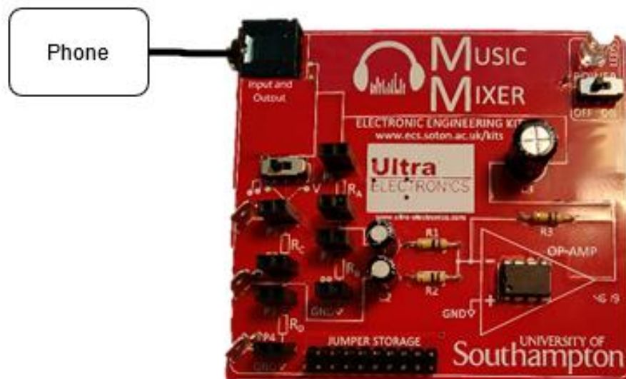
Figure 88: Use case of the board redesign with TRRS connection to a single phone that is used as both oscilloscope and signal generator
