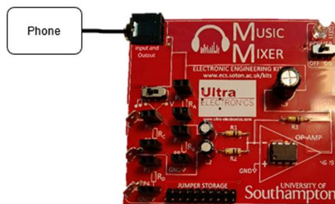
Figure 15: Mock-up of the board redesign with TRRS connection to a single phone that is used as both oscilloscope and signal generator
