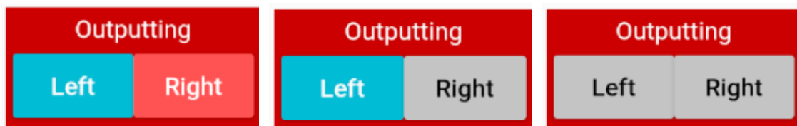
Figure 43: Outputting box with (Left) both signals turned on (Middle) left signal turned on (Right) none turned on
